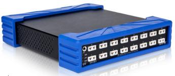
The EX1401 delivers accurate and highly repeatable thermocouple (±0.20°C) and voltage measurements by implementing fully integrated signal conditioning, 24-bit ADC's, and independent Cold Junction Compensation (CJC) on a per-channel basis.
