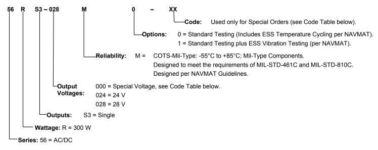
**Example:** 56RS3-028M0-01 = AC/DC; 300 Watt; Single Output; 28 V; COTS-Mil-Type; Standard Testing; Current Share
